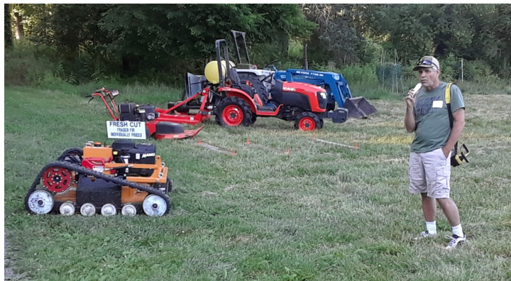
Fred Castenschiold demonstrates the "Alamo Ridge Runner" remote-controlled mower, used for mowing steep hillsides and wetlands such as in detention basins at the June twilight meeting.
